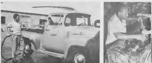
IMPORTANT DEN e Garage's constant fight against corrosion is keeping vehicles regularly washed to cut the salt spray. Employee here is R. Tromp. IMPORTANTE DEN e lucha constante di garage contra corrosión ta tene autonnan constantemente laba pa reduci e spartimento di salpeter. E empleado aki ta E. Tromp.
